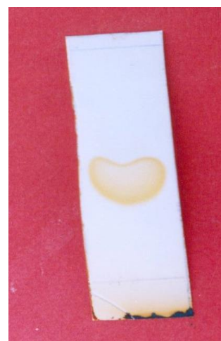
Fig. 2. TLC Test of purity alkaloid isolated from H. aureus in NH 4 OH: Me OH(3:200) by dragendorff
