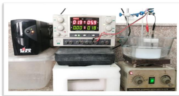
Fig. 1. The electrochemical system for preparation of Al 2 O 3 NPs
